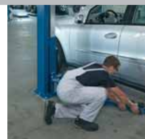
Telescopic lifting arms and lowest lifting point
