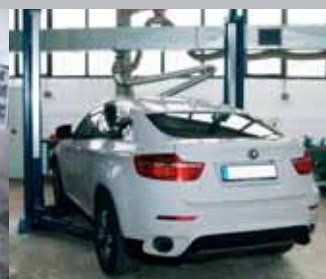
POWER LIFT HL 2.40 NT – Lift for passenger cars and transporter, for universal application
