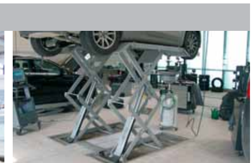
JUMBO LIFT NT 4000 – lifting vehicle from VW T5 with short wheelbase and similar vehicles | In-ground installation
