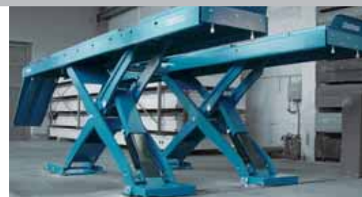
No fixed connection between the scissors
