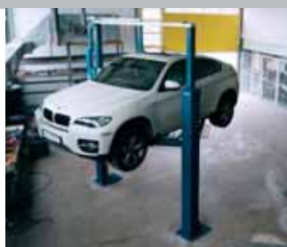
POWER LIFT HL 2.40 NT – Lift for passenger cars and transporter, for universal application
