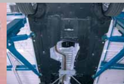
POWER LIFT HL 2.30 NT DT – short lifting arm with 2-times telescopic arms provide more adjustable range and simplifies lifting of shorter and wider vehicles
