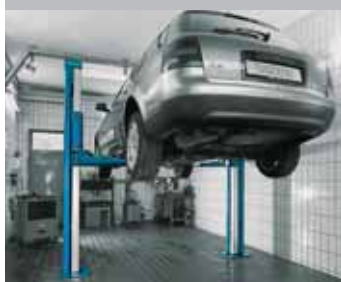
SMART LIFT 2.30 SL – lift for vehicles up to VW T5 with short wheelbase and similar vehicles
