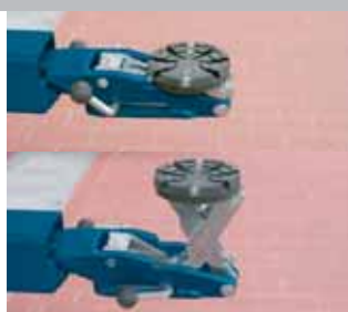
MINI MAX lifting arms easy and convenient to lift lowered vehicles and for cars with pressed side skirts
