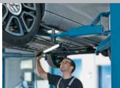
SMART LIFT 2.30 SL DT – short lifting arm with 2-times telescopic provides more adjustable range and simplifies lifting of shorter and wider vehicles
